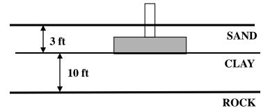
Solution: Since the water can't drain into rock the longest path is into the sand on the top, so the water molecule at the bottom of the clay layer will have to travel the 10 ft to the sandy soil. H = 10 ft.
