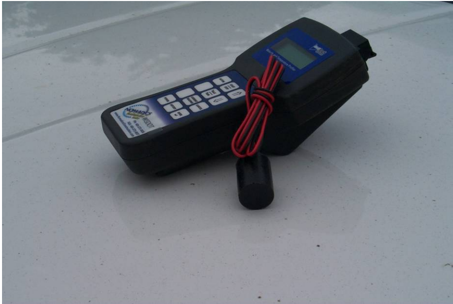
Figure 6. IntelliRock™ maturity reader and logger.
