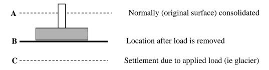
It is pretty intuitive that the stress applied to the soil (weight of the footing and the load the foot distributes) depends on the rates and distance of settlement. However, it is important to note that the decrease void ratio vs stress applied depends on if the footing is in the overconsolidated region or in a virgin area where the clay soil has never been consolidated there before. Review the diagram below for an example.
