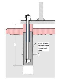
Example: Consider the below anchoring system. The bond between the anchor shaft and stone is 375 psi. The Diameter of the shaft is 8 inches and 15 feet long. What is the force that results in failure.
